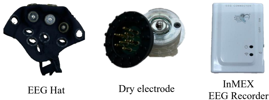
Fig. 1. The eight-channel wireless EEG system. The system comprises three components: (a) The EEG hat, (b) The dry EEG electrode used to mount on the EEG hat, and (c) The eight-channel InMEX EEG recorder.
